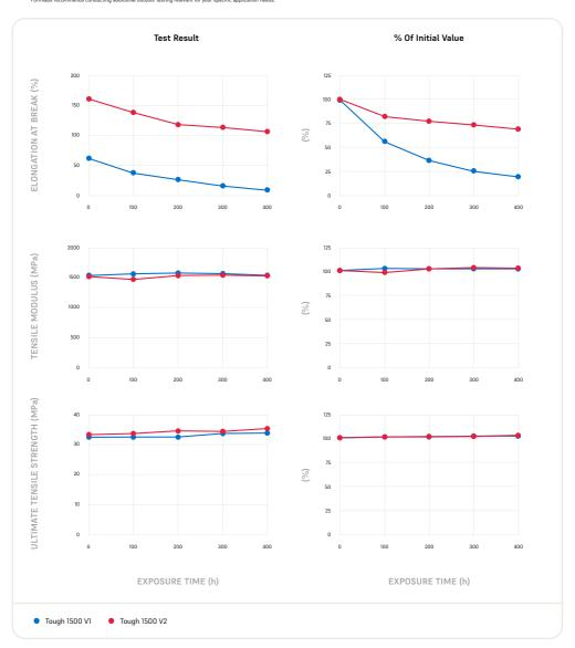
ASTM D432°. Cycle A for general applications, QUV/se, UNA 340 nm, 0.89 W/m²-nm, 8 hours UN light at 60°C followed by 4 hours at 50°C condensation in the dark. To reduce any sample warpage during test time samples were placed in tailor-made holders without any fixation clamps or mechanical load. Exposed samples were always removed from QUV before next condensation cycle to avoid samples that are soaked excessively with water before testing.
